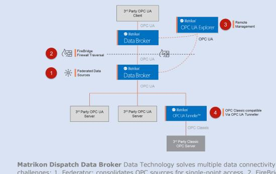
**Matrikon Dispatch Data Broker** Data Technology solves multiple data connectivity challenges: 1. Federator: consolidates OPC sources for single-point access. 2. FireBridge: enables secure connectivity while keeping in-bound firewall ports closed.3. Remote Management makes it easy to manage all Data Broker nodes. 4. Matrikon OPC UA Tunneller enables access to OPC Classic components.
